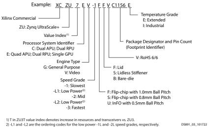
Figure 3: Zynq UltraScale+ MPSoC Ordering Information
