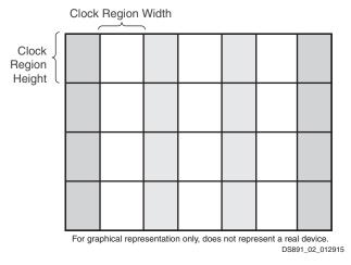
Figure 2: Column-Based Device Divided into Clock Regions
