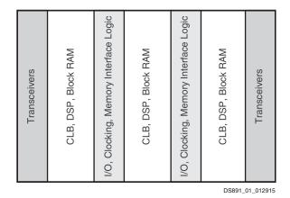
Figure 1: Device with Columnar Resources
