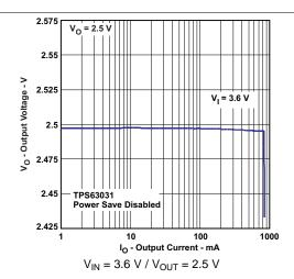
Figure 17. Output Voltage versus Output Current, TPS63030, Power-Save Disabled
