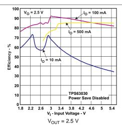
Figure 13. Efficiency versus Input Voltage, TPS63030, Power-Save Disabled
