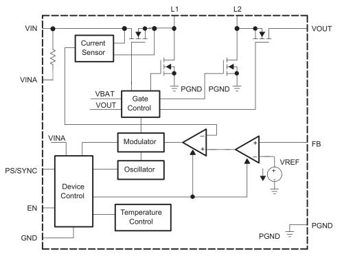
Figure 3. Functional Block Diagram (TPS63030)
