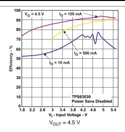
Figure 14. Efficiency versus Input Voltage, TPS63030, Power-Save Disabled
