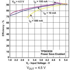
Figure 12. Efficiency versus Input Voltage, TPS63030, Power-Save Enabled
