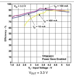
Figure 15. Efficiency versus Input Voltage, TPS63031, Power-Save Enabled
