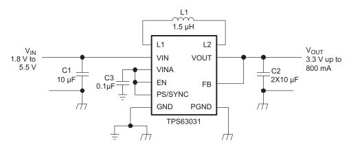
Figure 6. Typical Application Circuit for 3.3-V Fixed Output Voltage Option
