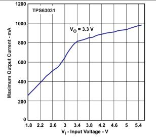
Figure 2. Maximum Output Current versus Input Voltage, TPS63031
