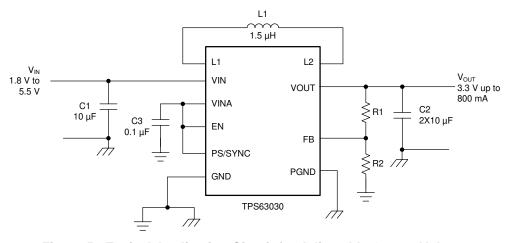
Figure 5. Typical Application Circuit for Adjustable Output Voltage
