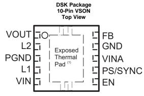
(1) The exposed thermal pad is connected to PGND.
