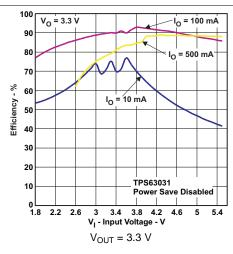
Figure 16. Efficiency versus Input Voltage, TPS63031, Power-Save Disabled
