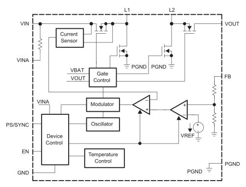
Figure 4. Functional Block Diagram (TPS63031)
