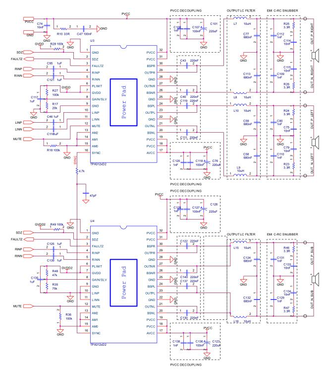
Figure 36. TPA312xD2 Schematic
