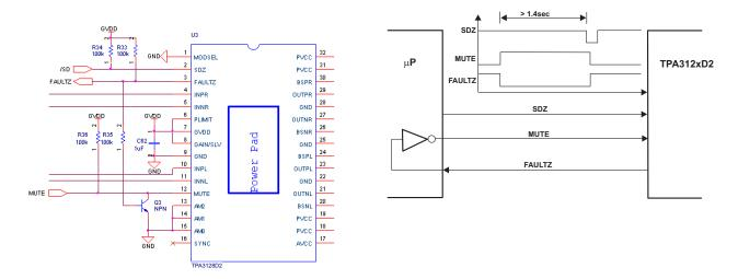
Figure 28. MUTE Driven by Inverted FAULTZ
