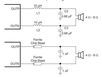
Figure 33. TPA31xxD2 Output Filters
