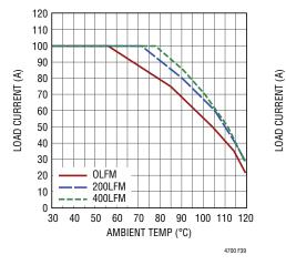
Figure 39. 5V to 0.8V Derating Curve, No Heat Sink
