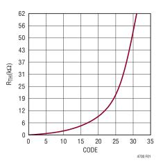
Figure 1. Programmable R<sub>COMP</sub>
