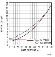
Figure 38. 1.8V Power Loss Curve
