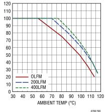
Figure 40. 12V to 0.8V Derating Curve, No Heat Sink
