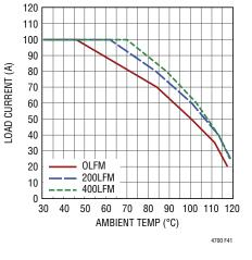
Figure 41. 5V to 1.2V Derating Curve, No Heat Sink
