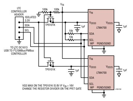
Figure 30. Controller Connection
