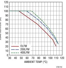
Figure 43. 5V to 1.8V Derating Curve, No Heat Sink
