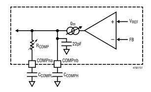
Figure 27. Programmable Loop Compensation
