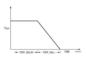
Figure 26. TOFF\_DELAY and TOFF\_FALL
