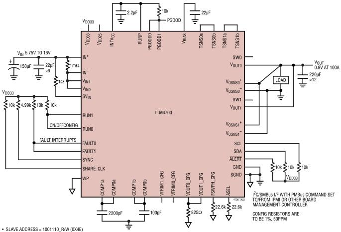
100A, 0.9V Output DC/DC µModule Regulator with I<sup>2</sup>C/SMBus/PMBus Serial Interface
