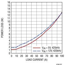
Figure 37. 1.2 Power Loss Curve
