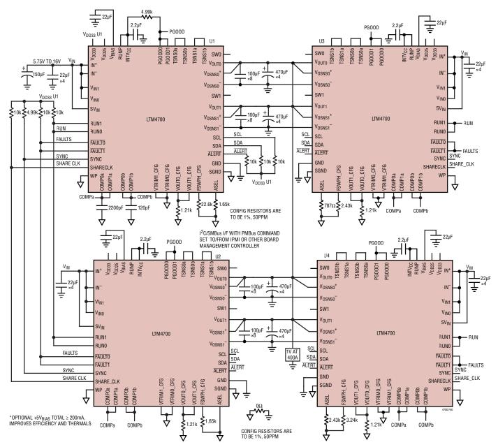
Figure 50. 8-Phase Operation with Four LTM4700 Producing 1V at 400A. Power System Management Features Accessible Through LTM4700 Over 2-Wire I<sup>2</sup>C/SMBus/PMBus Serial Interface
