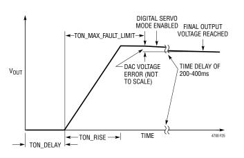
Figure 25. Timing Controlled V<sub>OUT</sub> Rise
