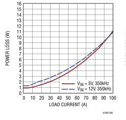
Figure 36. 0.8V Power Loss Curve
