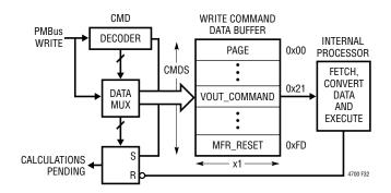
Figure 32. Write Command Data Processing
