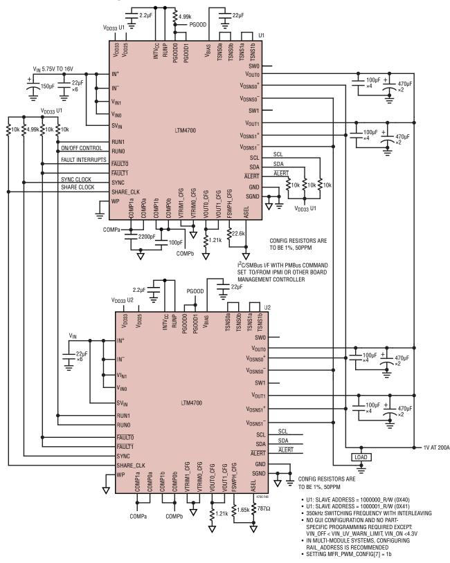
Figure 48. Two Paralleled LTM4700 Producing 1V<sub>OUT</sub> at 200A. Integrated Power System Management Features Accessible Over 2-Wire I<sup>2</sup>C/SMBus/PMBus Serial Interface
