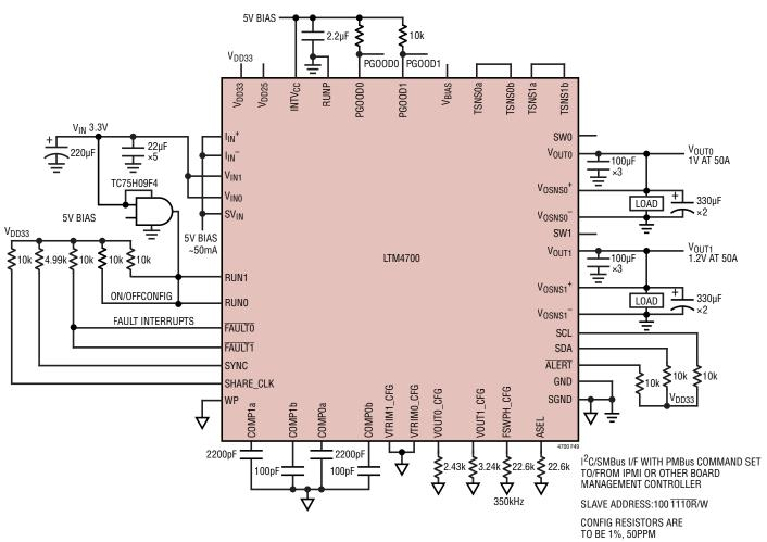
Figure 49. 3.3V Input LTM4700 Producing  $1V_{OUT}$  and  $1.2V_{OUT}$  at Up to 50A. Integrated Power System Management Features Accessible Over 2-Wire I<sup>2</sup>C/SMBus/PMBus Serial Interface
