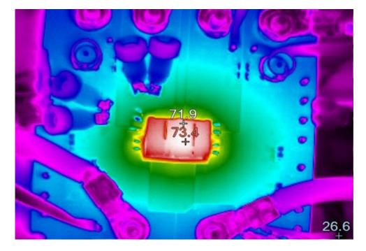
Figure 35. Thermal Image, LTM4700 Running from 12V Input to 1V Output, 100A Output with 200LFM Airflow, No Heat Sinking
