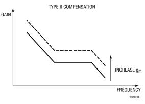
Figure 28. Error Amp g<sub>m</sub> Adjust
