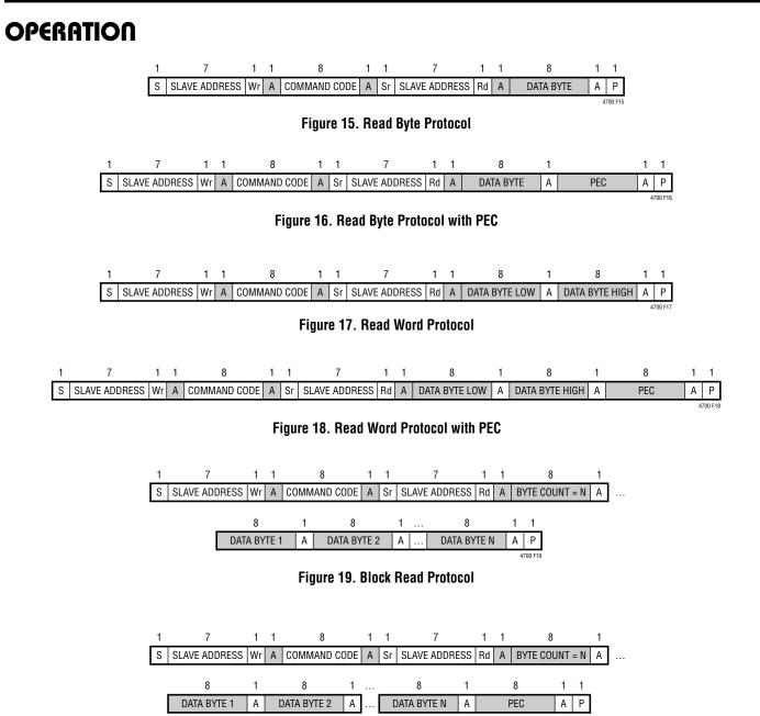
Figure 20. Block Read Protocol with PEC
