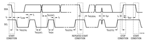
Figure 6. PMBus Timing Diagram
