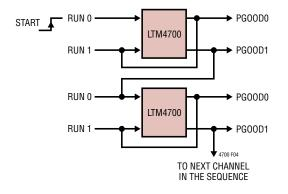
Figure 4. Event (Voltage) Based Sequencing
