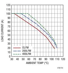
Figure 44. 12V to 1.8V Derating Curve, No Heat Sink
