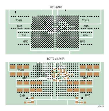
Figure 45. Recommended PCB Layout Package Top View
