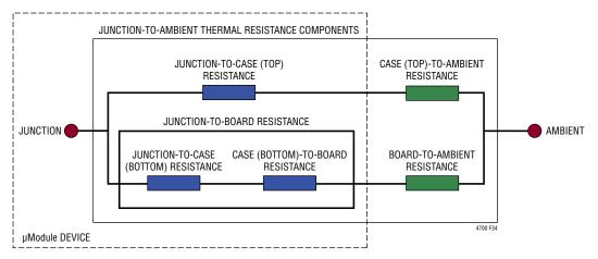
Figure 34. Graphical Representation of JESD51-12 Thermal Coefficients
