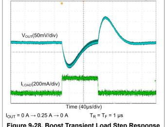
Figure 9-28. Boost Transient Load Step Response
