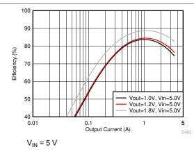
Figure 9-5. Buck Efficiency in Forced PWM Mode
