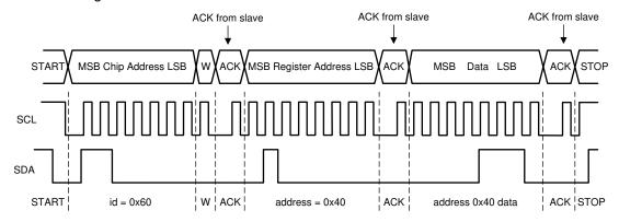
Figure 8-18. Write Cycle (w = write; SDA = 0), id = Device Address = 60Hex for LP87702-Q1
