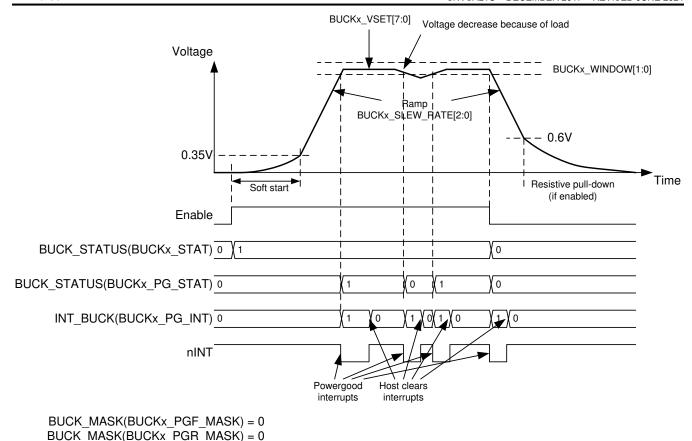
Figure 8-4. Buck Converter Enable and Disable
