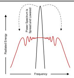
Where a fixed frequency converter exhibits large amounts of spectral energy at the switching frequency, the spread spectrum architecture of the LP87702-Q1 spreads that energy over a large bandwidth.
