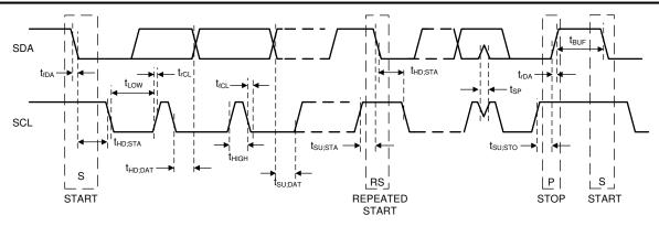
Figure 8-17. I<sup>2</sup>C-Compatible Timing
