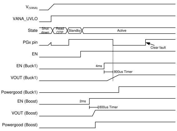
Figure 8-10. PGx Pin Operation in Gated Mode.
