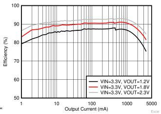
**Buck Efficiency vs Output Current**
