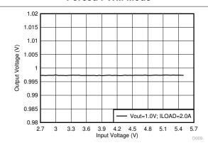
Figure 9-7. Buck Output Voltage vs Load Current in | Figure 9-8. Buck Output Voltage vs Input Voltage in **PWM Mode**
