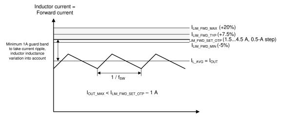
Figure 9-2. Current Limit vs Maximum Output Current
