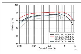
Figure 9-3. Buck Efficiency in AUTO (PFM/PWM) Mode
