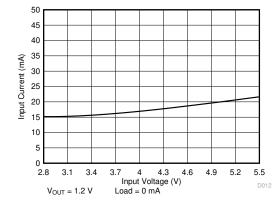
Figure 7-5. Active State Current Consumption vs Input Voltage, One Buck Converter Enabled in PWM Mode
