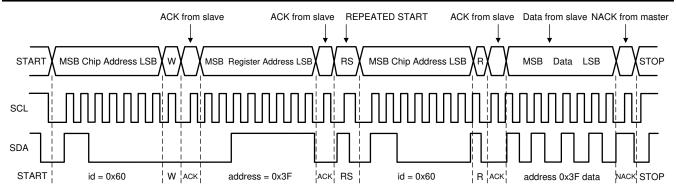
A WRITE function must precede the READ function as shown above when the READ function is accomplished.
