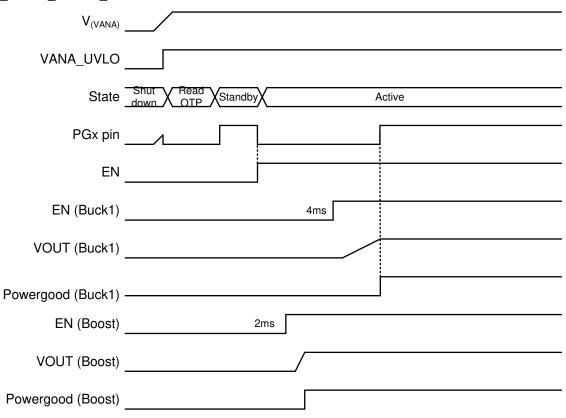
Figure 8-11. PGx Pin Operation in Continuous Mode
