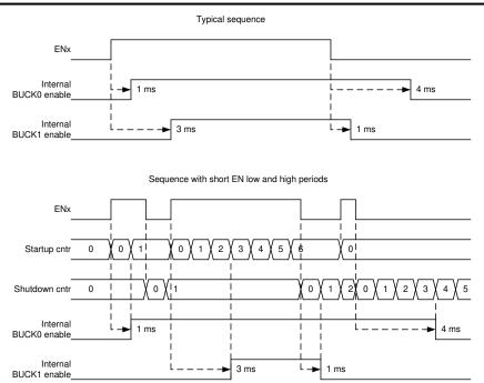
Figure 8-7. Start-up and Shutdown Sequencing Example
