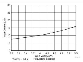
Figure 7-3. Standby Current Consumption vs Input Voltage
