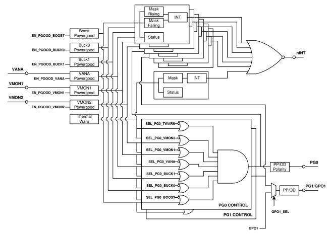
Figure 8-9. Block Diagram of Power-Good Connections
