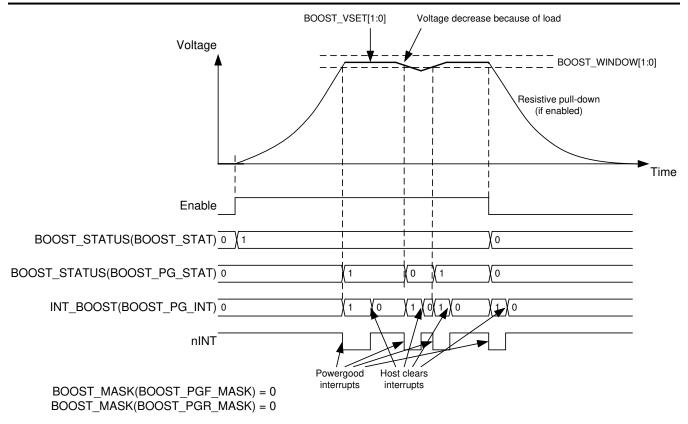
Figure 8-5. Boost Converter Enable and Disable
