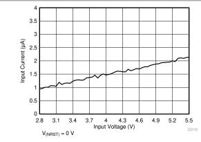
Figure 7-2. Shutdown Current Consumption vs Input Voltage
