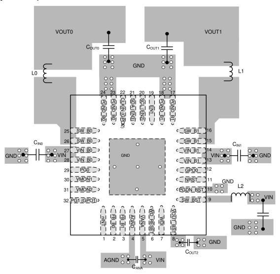
Figure 11-1. LP87702-Q1 Board Layout Example
