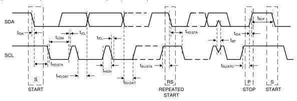
Figure 7-1. I<sup>2</sup>C Timing
