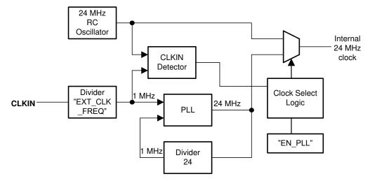
Figure 8-3. Clock and PLL Module
