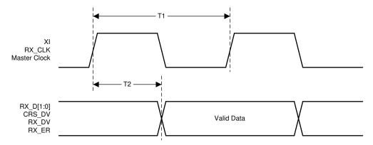
Figure 7-10. RMII Receive Timing
