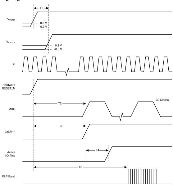
Figure 7-1. Power-Up Timing
