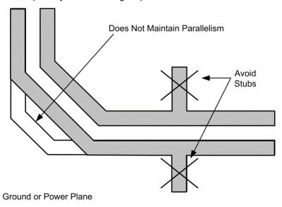
Figure 11-1. Differential Signal Traces
