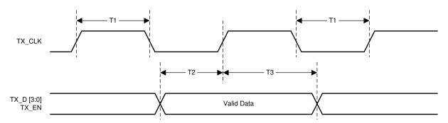
Figure 7-7. 10-Mbps Transmit Timing
