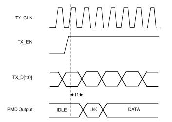
Figure 7-16. 100BASE-TX Transmit Latency Timing
