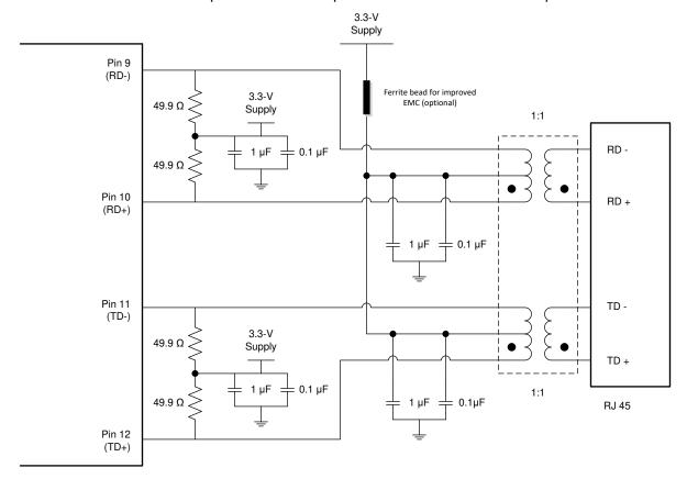
Figure 9-2. TPI Network Circuit
