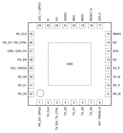
Figure 6-1. RHB Package 32-Pin VQFN Top View
