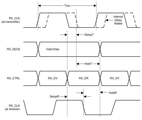
Figure 7-12. RGMII Receive Timing
