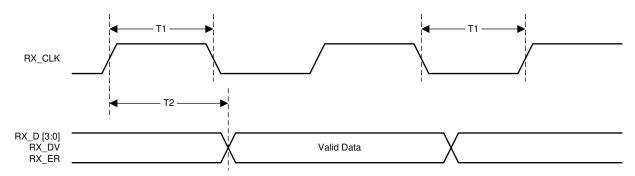
Figure 7-8. 10-Mbps Receive Timing
