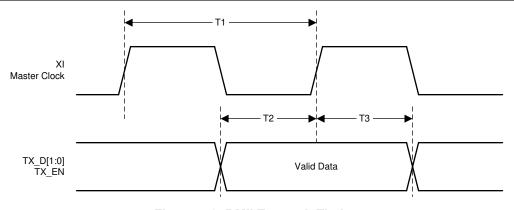
Figure 7-9. RMII Transmit Timing
