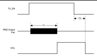
Figure 7-15. 10BASE-Te Jabber Timing
