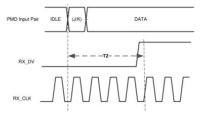
Figure 7-17. 100BASE-TX Receive Latency Timing
