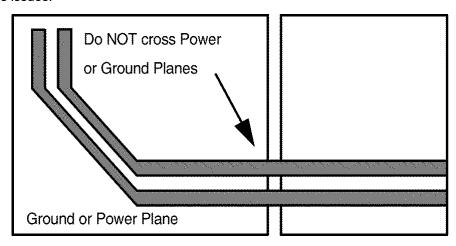
Figure 11-2. Differential Signal Pair and Plane Crossing
