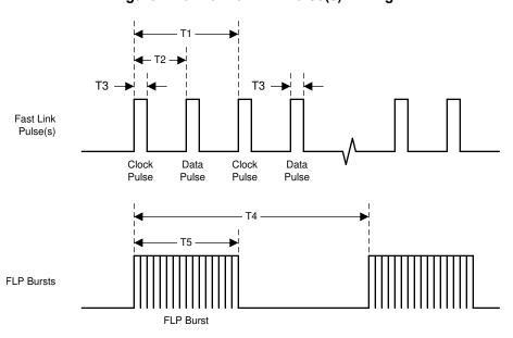
Figure 7-14. Fast Link Pulse Timing
