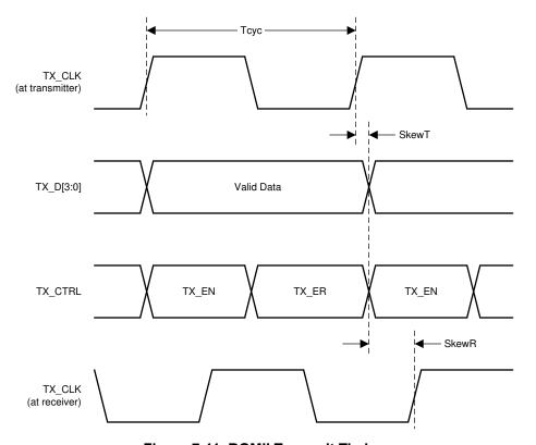
Figure 7-11. RGMII Transmit Timing
