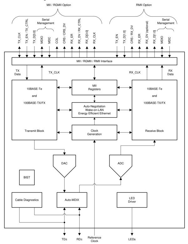
Figure 8-1. DP83822 Functional Block Diagram
