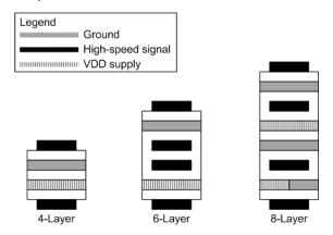
Figure 11-3. Recommended Layer Stack-Up
