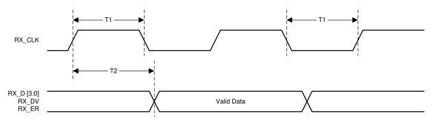
Figure 7-6. 100-Mbps Receive Timing
