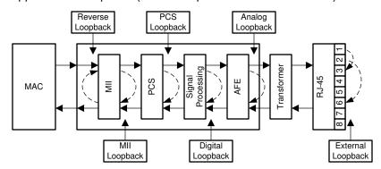
Figure 8-8. Loopback Test Modes
