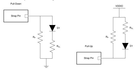
Figure 8-11. Example Strap Connections
