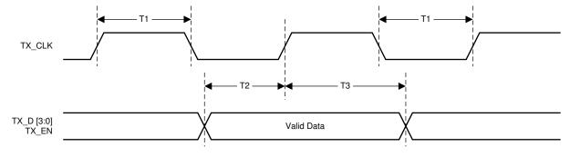
Figure 7-5. 100-Mbps Transmit Timing
