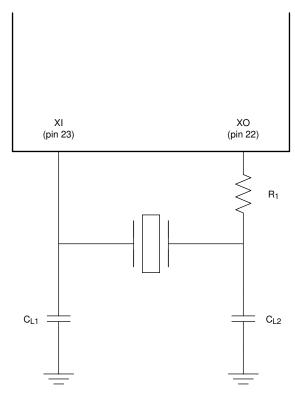
Figure 9-4. Crystal Oscillator Circuit
