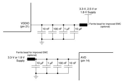
A. The smallest value is placed closest to the pin
