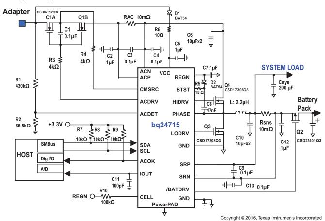
Fs = 800kHz,  $I_{ADPT}$  = 3.0A,  $I_{CHRG}$  = 2.944A,  $I_{SYSTEM}$  = 5A,  $V_{CHRG}$  = 12.592V, 65W adapter and 3S2P battery pack Csys : 200  $\mu$ F is lumped system bus capacitance
