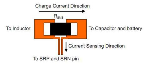
Figure 21. Sensing Resistor PCB Layout
