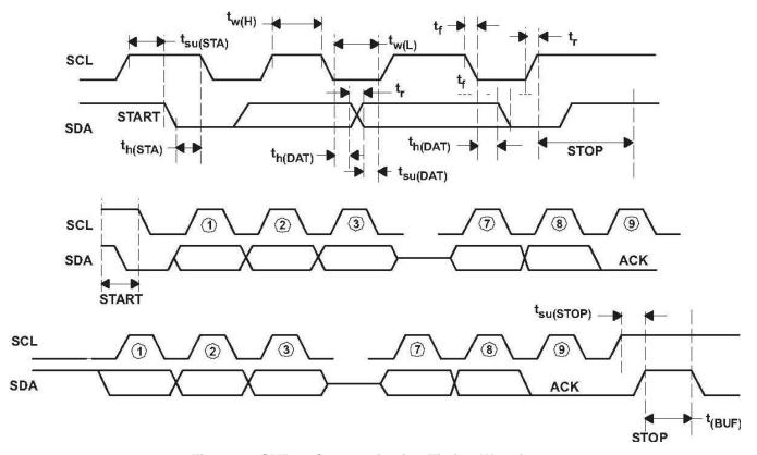
Figure 1. SMBus Communication Timing Waveforms
