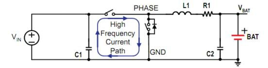
Figure 20. High Frequency Current Path
