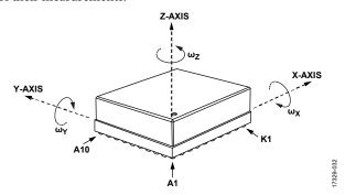
Figure 49. Gyroscope Axis and Polarity Assignments
