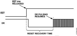
Figure 39. Data Ready Response During Reset ( $\overline{RST} = 0$ ) Recovery
