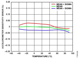
Figure 26. Accelerometer Sensitivity Error vs. Temperature, Cold to Hot, All Axes
