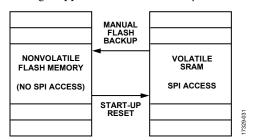
Figure 48. SRAM and Flash Memory Diagram
