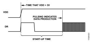
Figure 37. Data Ready Response During Startup
