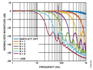
Figure 29. Accelerometer Normalized Noise Density
