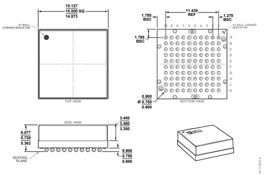
Figure 67. 100-Ball Ball Grid Array Module [BGA] (ML-100-1) Dimensions shown in millimeters
