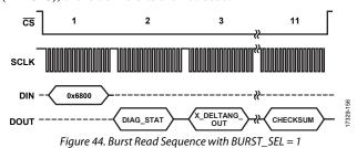
The sequence of registers (and checksum value) in the burst read includes the following registers and value: DIAG\_STAT, X\_DELTANG\_OUT, Y\_DELTANG\_OUT, Z\_DELTANG\_OUT, X\_DELTVEL\_OUT, Y\_DELTVEL\_OUT, Z\_DELTVEL\_OUT, TEMP\_OUT, DATA\_ CNTR, and the checksum value.
