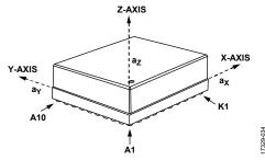
Figure 51. Accelerometer Axis and Polarity Assignments
