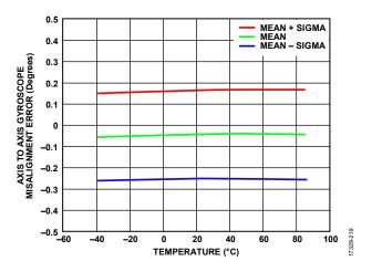
Figure 19. Axis to Axis Gyroscope Misalignment Error vs. Temperature, All Axes, ADIS16507-1
