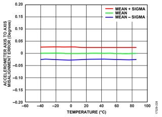
$\textit{Figure 28. Accelerometer Axis to Axis Misalignment Error vs.} \ \textit{Temperature}$
