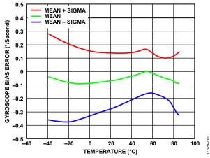
Figure 10. Gyroscope Bias Error vs. Temperature, ADIS16507-1, All Axes
