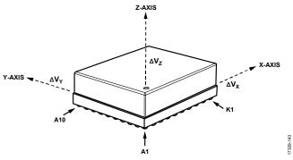
Figure 55. Delta Velocity Axis and Polarity Assignments
