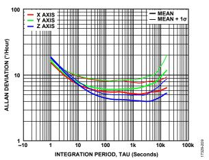
Figure 9. Gyroscope Allan Deviation,  $T_C = 25^{\circ}C$ , ADIS16507-3, Plot Taken After 10 Hours of Settling Time
