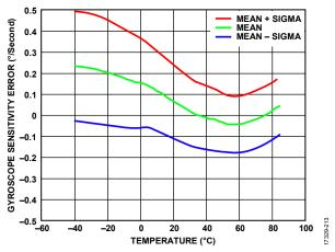
Figure 13. Gyroscope Sensitivity Error vs. Temperature, ADIS16507-1,
